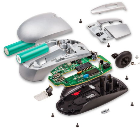
9 Explode View of Wireless Mouse
